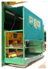
The SU300DP is a compact desilter with a discharge pump. It is designed to work downstream of "SUPERCLEAN", а "SS" desanding unit or other suitable desander in civil engineering, slurry shield tunnelling directional drilling applications and will process flowrates of up to 300m<sup>3</sup>/hr. The unit will separate sands and medium silts from bentonite fluid having a Marsh Funnel viscosity of less than 100 seconds per U.S. Quart. The SU300DP consists of two modules that are joined together for
